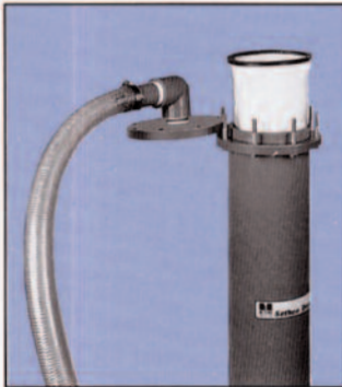
Filter bags are easy to replace. 1. Remove cover. 2. Pull out used filter bag. 3. New filter bag fits quickly and securely into chamber.
